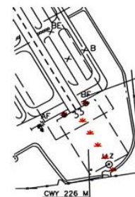
RWY 33 STROBOSCOPIC FLASHING APPROACH LIGHTS
